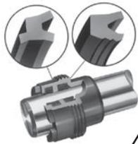
**"Jewel" Rod Gland Assembly –** Externally removable without cylinder disassembly. Long bearing surface is inboard of the seals, assuring positive lubrication from within the cylinder. An "O" ring is used as a seal between gland and head, and also serves as a prevailing torque-type lock.
